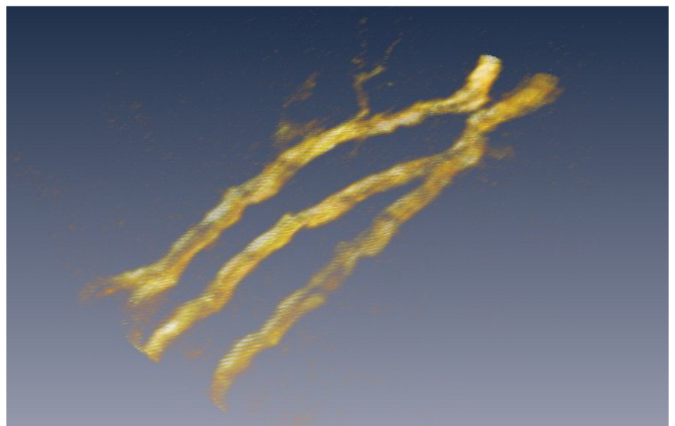
Optoacoustic image of vessels in a human forearm generated with DiPhAS and a Nd:YAG laser
