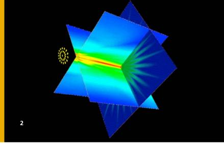
elements which are then assembled to get the complete solution. Finally the vibrational shape of the ultrasonic transducer is visualized and optimized.
