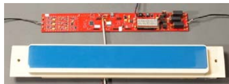
IBMT 3-frequency sidescanner (electronic is normally pressure-tolerantly integrated in transducer).
