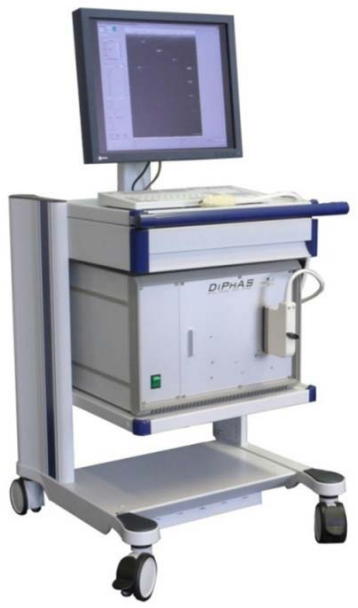
Macroscopic optoacoustic imaging system based on DiPhAS.
