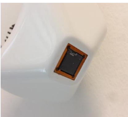
2.5 MHz matrix array with 1024 transducer elements, pitch 308 \mu\text{m}
