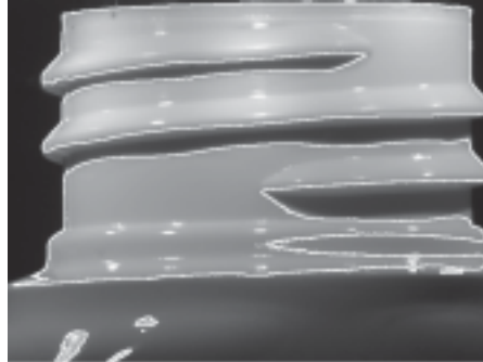
Figure 1: Edge detection after captured image was processed. Edges are used for the estimation of some of the neck parameters.
