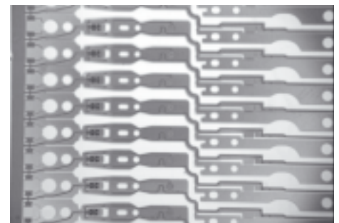
Machine Vision image of bonding pads on printed circuit boards for defect detection.
