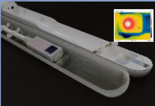
Small animal applicator with integrated ultrasound matrix array transducer (left) and its pressure distribution using volumetric beam steering (right)
